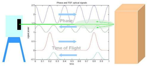
Figure 2. Working principle of phase based and time-of-flight laser scanners (from California Department of Transportation, 2011)
