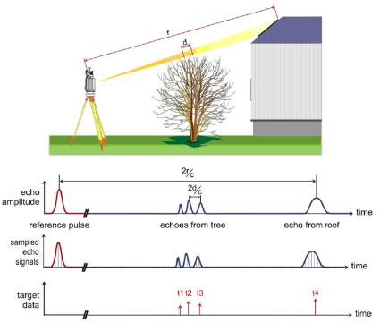
Figure 4. Working principle of waveform processing laser scanners (from Ullrich & Pfennigbuer, 2011)
