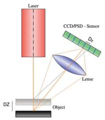
Figure 3. Working principle of triangulation based laser scanners (from Lee & Xu, 2009)
