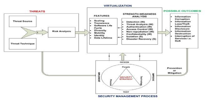
Figure 2. Proposed virtualization security model
