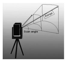
Figure 1. Principle of Terrestrial Laser Scanning; from measured range and scan angle combined with position and orientation of the scanner the three-dimensional coordinates of the points hit by laser beams can be computed, resulting in a point cloud of 3D coordinates (from Lemmens, 2011).
